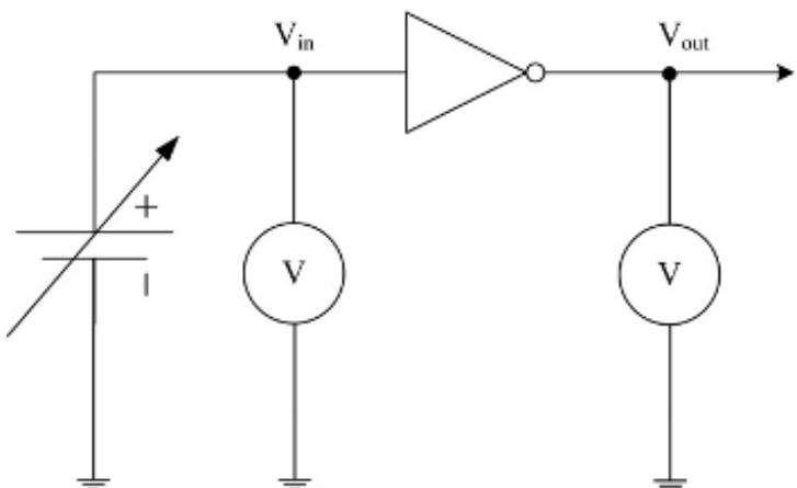
*Merits:* Directly connecting the voltage source to the IC input is not recommended as the absolute maximum rating of the input may accidentally be exceeded causing device permanent damage.
