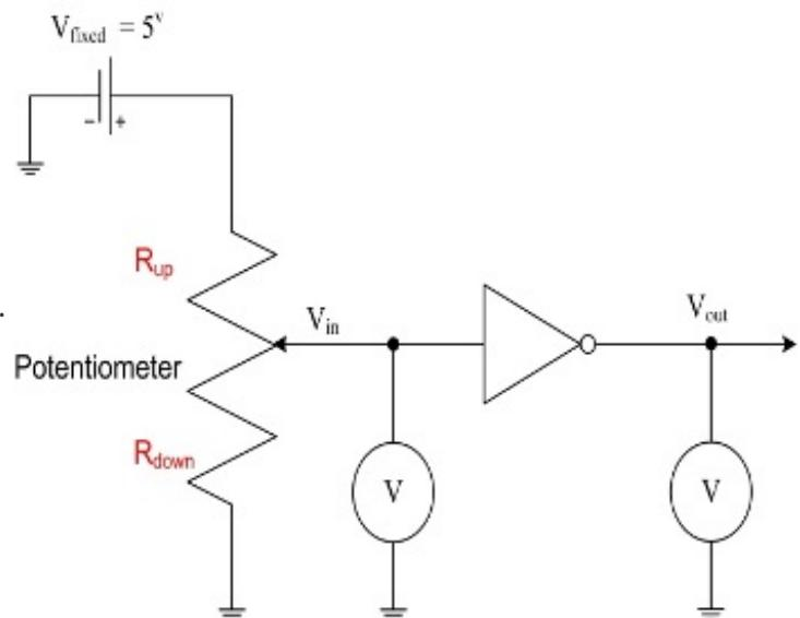
*Merits:* If  $R_{up} \approx 0$ , direct connection of the voltage source to the IC input may cause an input voltage overshoot and is not recommended.
