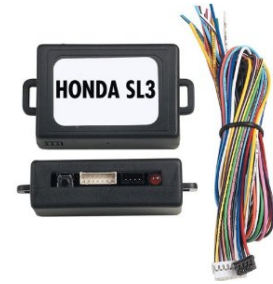
Figure 9 'Honda-SL3' immobilizer bypasser by Fortin Electronics
