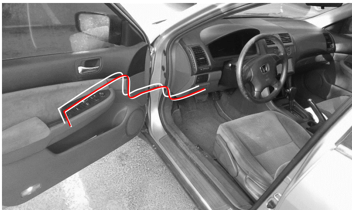
Figure 2 Location and extension of the security system control wirings
