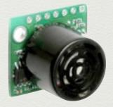
This sensors will be connected to Arduino to sense if a car is approaching.
