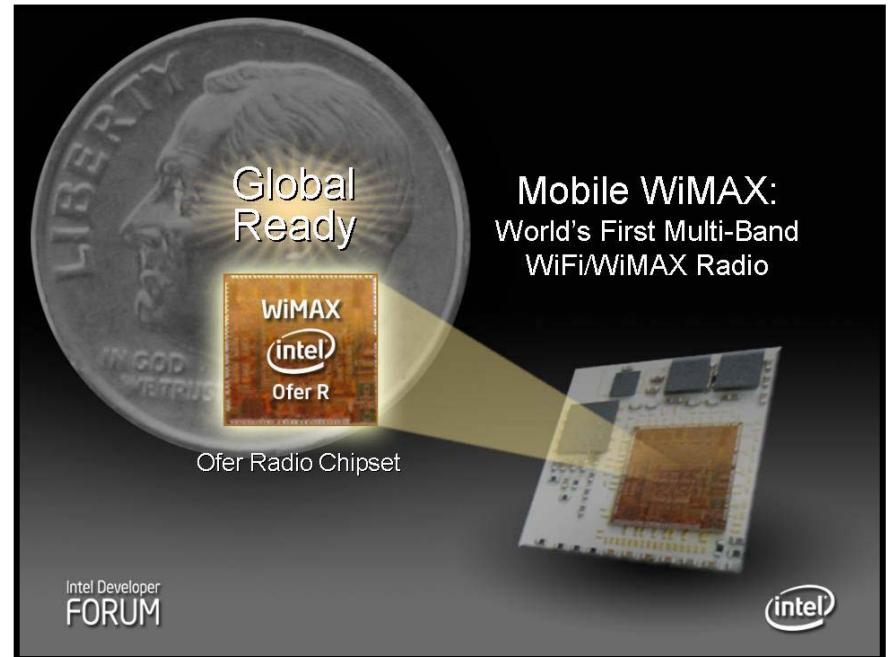
Offer-R: World's First Single Chip Wi-Fi / WiMAX Radio for Mobile Devices
