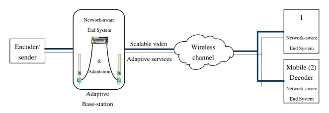
Fig. 2 System configuration for video streaming over cellular mobile network (Two subscriber's example)
