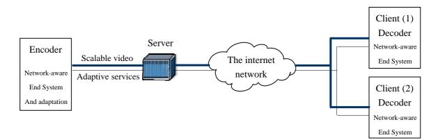
Fig. 1 System configuration for internet streaming of video (Two client's example)
