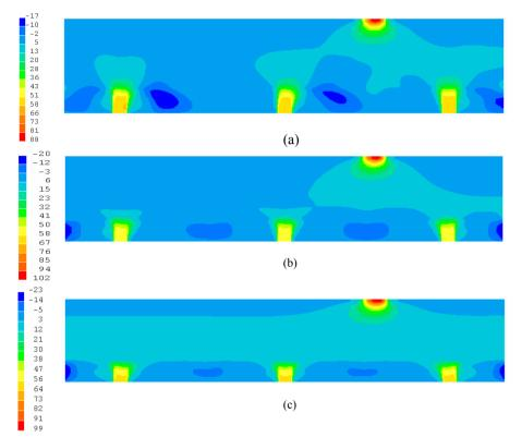
Figure 8. (a) Contour of W1 for the packed bed, and (b) Velocity Field for the packed bed. (a)  $(F_z = 10 \text{ and } F_y = 10)$ , (b)  $(F_z=100, F_y=10)$ , (c) $(F_z=5000, F_y=5000)$ .
