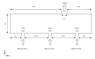
Figure 1. Schematic of the simulated vessel.
