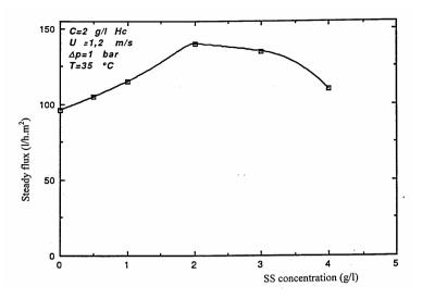
Figure 3: Influence of SS concentration on steady flux
