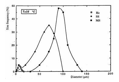
Figure 2: Size distribution of HC droplets, SS particles and MS particles
