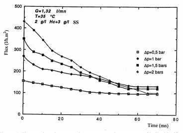
Figure 6: Flux against time at various pressures in presence of helical baffles
