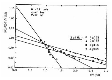
Figure 5: Flux modeling, 2 g/l HC and variable SS concentration
