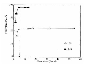
Figure 4: Permeate steady flux against shear stress, 2 g/l HC, 3 g/l SS, 35°C and 2 bars
