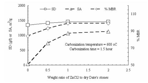
Figure 2: Effect of weight ratio of zinc chloride to dry dates' stones on % methylene blue removal blue (% MBR), solid density (SD) and specific surface area (SA) for activated carbons carbonized for 1.5 hour at 600 °C.
