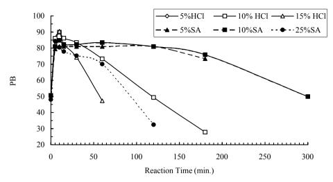
Figure 5: Effect of reaction time and acid (HCl or sulfuric acid (SA)) concentration on PB for clay deoiled by Petroleum ether at optimum conditions. WCR = 5; RPM =200; Temperature = Boiling.
