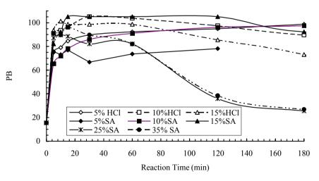
Figure 6: Effect of reaction time and acid (HCl or sulfuric acid (SA)) concentration on PB for clay deoiled by boil-off method at optimum conditions. WCR = 5; RPM =200; Temperature = Boiling.
