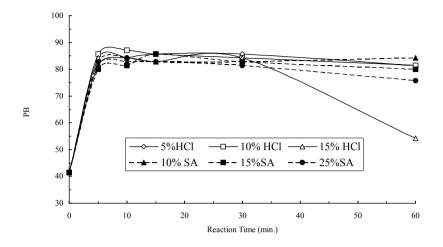
Figure 3: Effect of reaction time and acid (HCl or sulfuric acid (SA)) concentration on PB for clay deoiled by Acetone at optimum conditions. WCR = 5; RPM =200; Temperature = Boiling.
