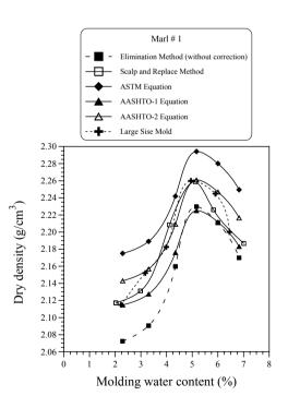
Figure 12. The moisture-density relationships for Marl # 1 using different correction methods
