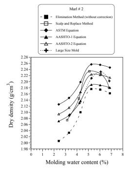
Figure 13. The moisture-density relationships for Marl # 2 using different correction methods
