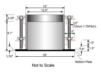
Figure 3. The large-size mold and accessories
