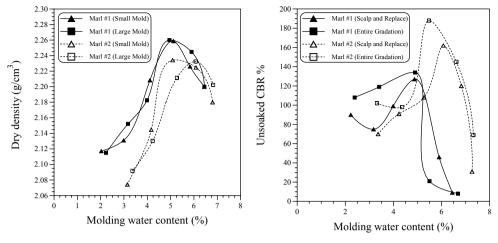
Figure 7. The moisture-density relationships for both marls using both molds
