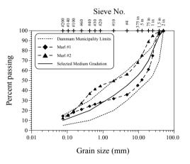
Figure 2. Grain size distribution of the collected materials and the selected gradation for the testing program
