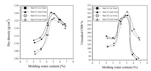
Figure 4. The moisture-density relationships for both marls using two trials
