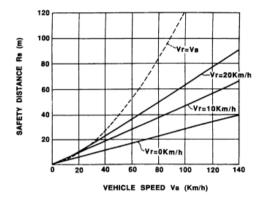
Fig. 1 Variation of safety distance with vehicle.
