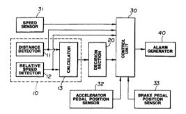
Fig. 2 Block diagram for excessive approach decision kit.
