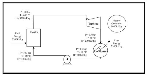
Figure-2: Cogeneration Cycle
