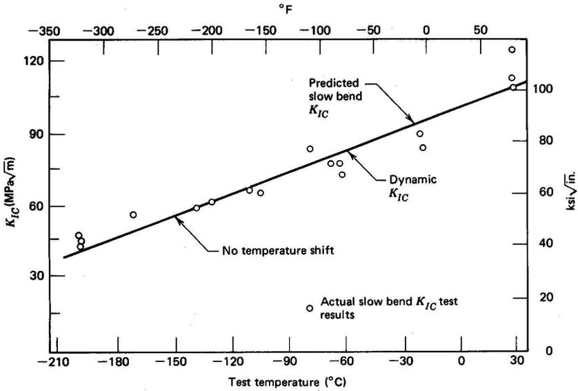
Figure-4 (b) Prediction of loading rate effect on  $K_{IC}$  for high-strength 18Ni (250) maraging steel with marginal strain-rate sensitivity [Barsom and Rolfe, 1970].
