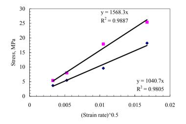
Figure 6. A linear plot of stress vs.  $\dot{\varepsilon}^{0.5}$  in region II for grain size 2.8  $\mu$ m( diamond) and 3.9  $\mu$ m ( square).
