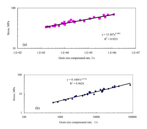
Figure 7. Flow stress vs. grain size compensated strain rate for (a) dislocation creep region, (b) superplastic region.
