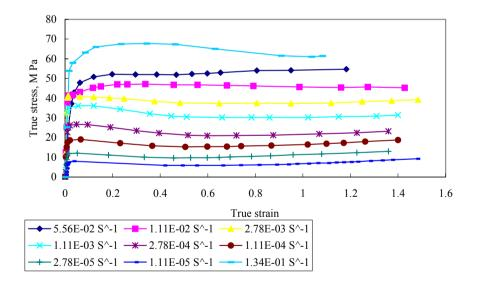
Figure 1. True stress-strain curves for  $d=2.8 \ \mu m$  (top) and  $d=5.0 \ \mu m$  (bottom).
