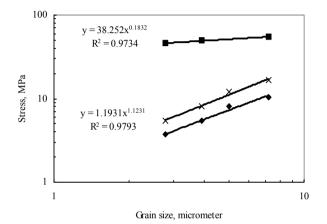
Figure 3. The relation between flow stress and grain size in region II (diamond,  $\dot{\epsilon} = 1.1 \times 10^{-5} \text{ s}^{-1}$ ; x,  $\dot{\epsilon} = 2.8 \times 10^{-5} \text{ s}^{-1}$ ; the value of s = 1.1) and region III (square,  $\dot{\epsilon} = 1.3 \times 10^{-2} \text{ s}^{-1}$ ; the value of s = 0.18).
