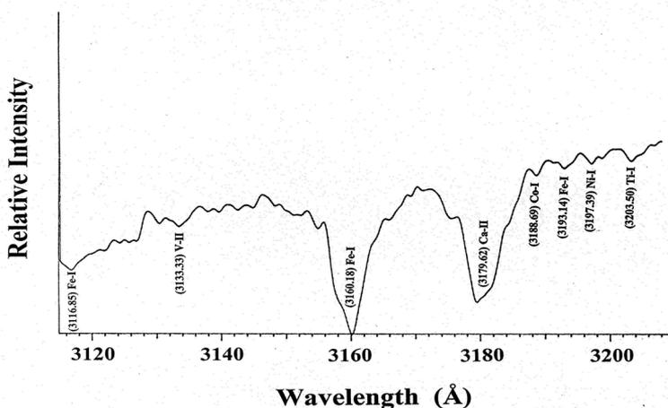
**Figure: 3** Typical spectrum recorded in the 3110- 3220 Å. Various elements present in the rock sample are indicated.
