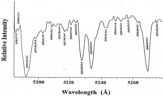
**Figure: 5** Typical spectrum recorded in the 5200 - 5280 Å. Various elements present in the rock sample are indicated.
