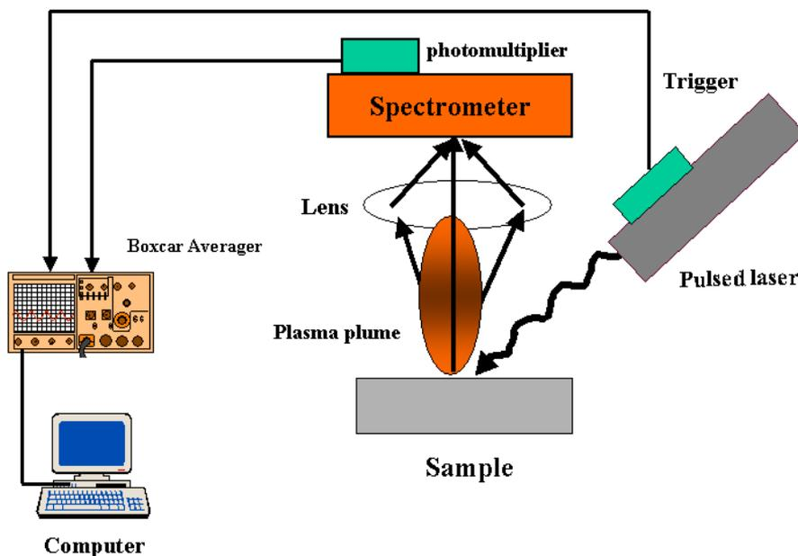
**Figure:1** Schematics of the experimental setup for the geological rock analysis
