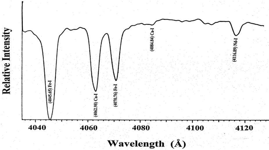
**Figure: 4** Typical spectrum recorded in the 4030- 4140 Å. Various elements present in the rock sample are indicated.
