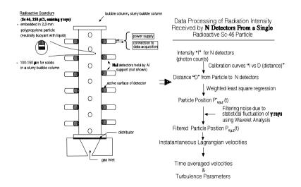
Figure 2: Schematic Diagram of CREL Computer Automated Radioactive Particle Tracking (CARPT)
