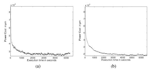
Fig. 9. Power-cost versus execution time: (a) OFSE and (b) AFSE.
