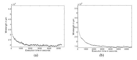
Fig. 8. Wire-length versus execution time: (a) OFSE and (b) AFSE.
