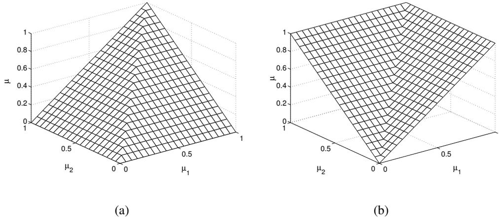
**Fig. 1.** (a) Fuzzy Min Operator. (b) Fuzzy Max Operator.
