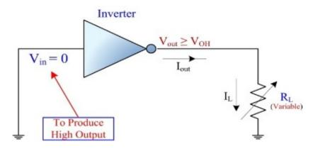
• For the highest impedance [3] load (open circuit), there will be no load (no current drawn, i.e.  $I_{out} = 0$ ), and  $V_{out}$  assumes its highest value.
