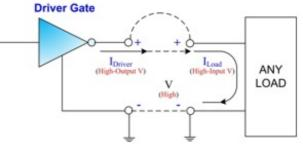
• When the *driver output* is low ( $V_{out} \le V_{OL}$ ), the maximum current that can be *sunk into* the driver from the load is designated as  $I_{OL}$ .
