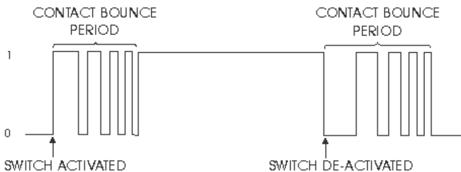
Figure 3. The Bouncing Problem of a Mechanical Switch
